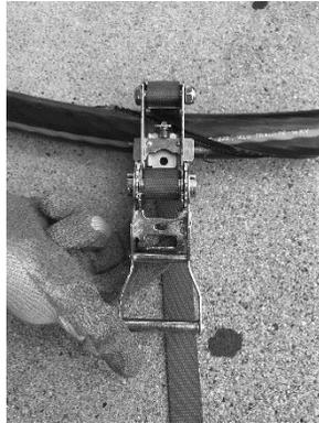
After you have completed the strip and you are holding THE RIPJACK™ by the handle, pull and hold the safety clamp's release tab (Figure 6). Open the ratchet buckle so it is completely open and flat (Figure 7).
